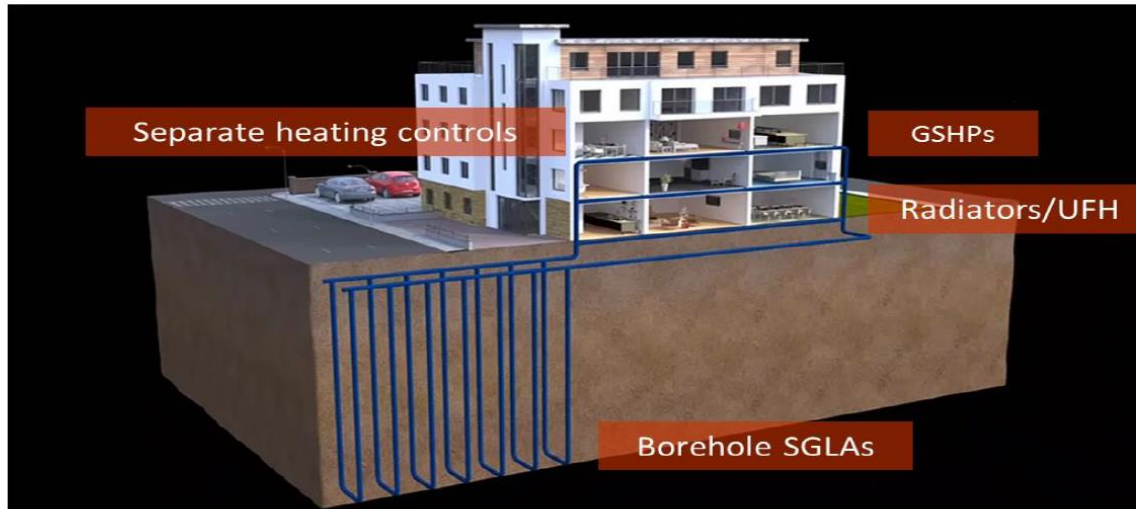
Figure 2 Schematic demonstrating the general design of a GSHP installation including the ground array.
